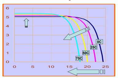
This characteristic is important in determining the dc voltage window of grid connected inverters
