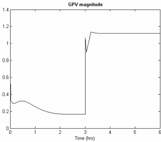
Figure 8. |GVP| for -20% bias volume sensor fault
