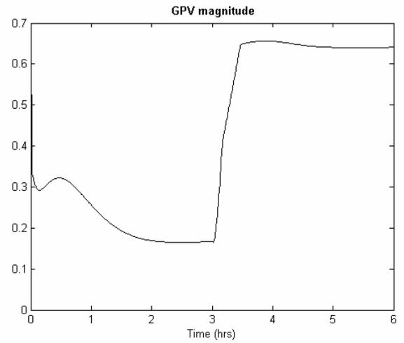
Figure 11. |GVP| for -20% bias outflow valve fault
