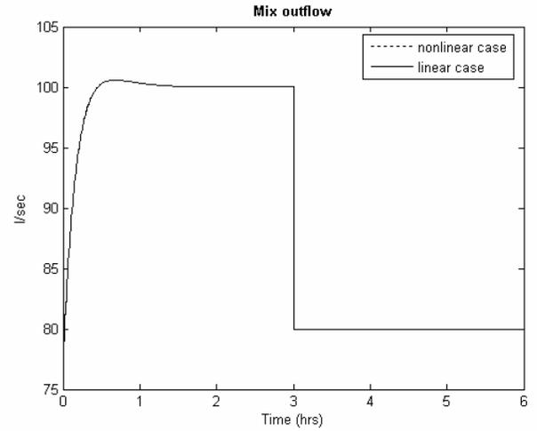
Figure 10. Outflow valve time-histories (-20% bias fault)
