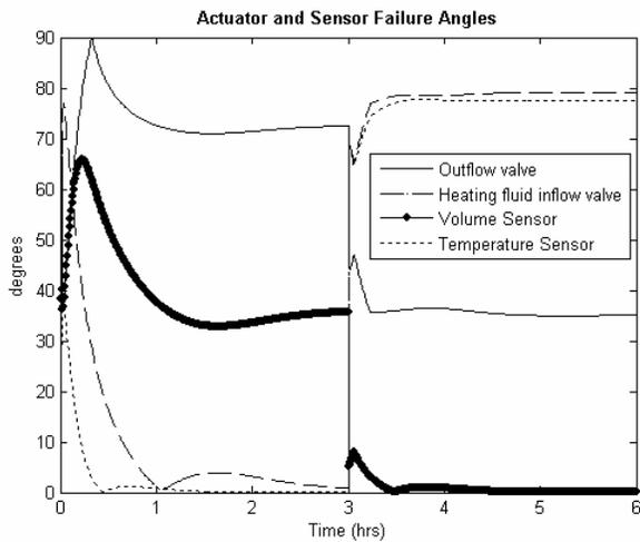
Figure 9. GVP angles for -20% bias volume sensor fault
