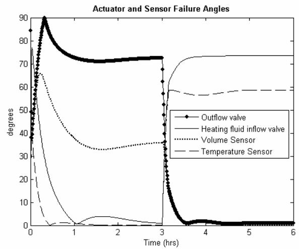
Figure 12. GVP angles for -20% bias outflow valve fault
