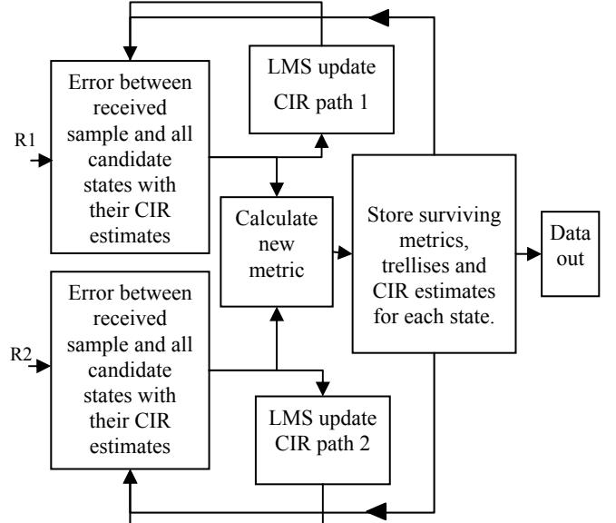
Figure 1. DSA flow diagram for two antenna diversity.
