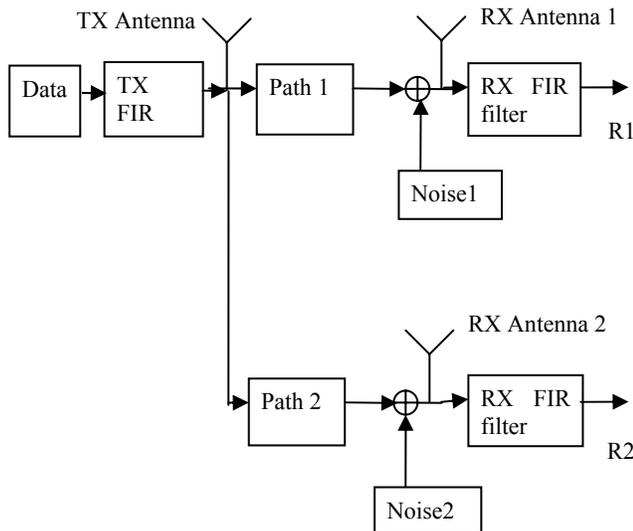
**Figure 2. Model of communication link.**
