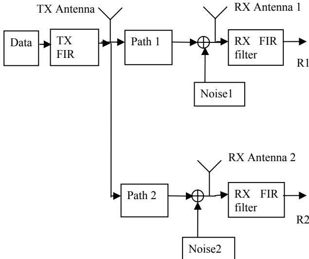
**Figure 2. Model of communication link.**
