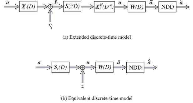
Fig. 5. Discrete-time model of the system.
