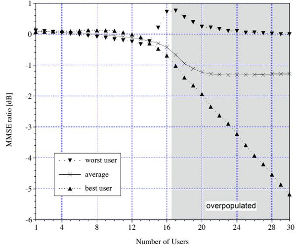
Fig. 13. Ratio of the MMSE between MNE-DDFE and MNP-DDFE over the number of system users.
