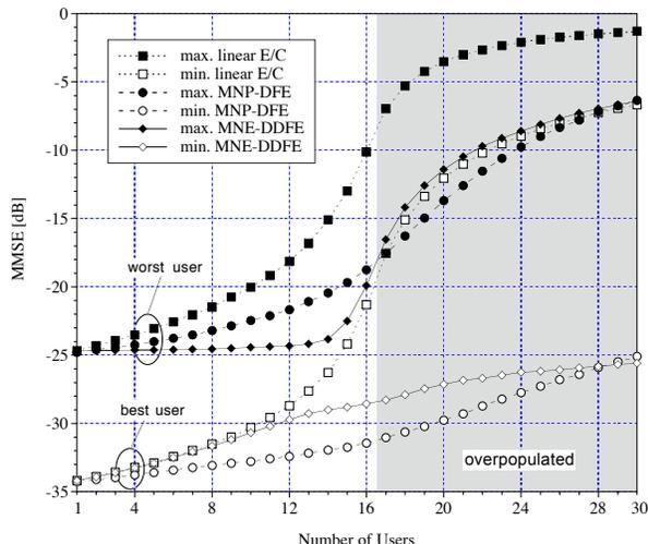
Fig. 11. MMSE for linear E/C, MNP-DFE and MNE-DDFE (received SNR's per user varying by up to 10 dB).
