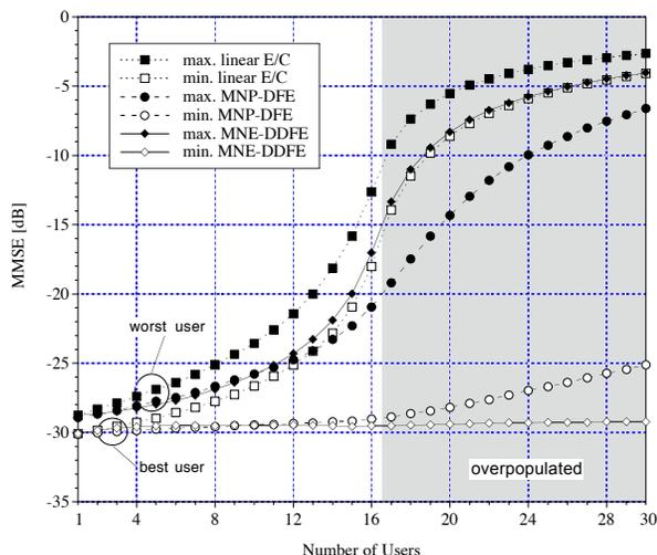
Fig. 12. MMSE for linear E/C, MNP-DFE and MNE-DDFE (received SNR's per user varying by up to 1 dB).
