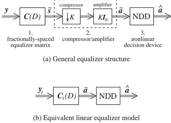
Fig. 2. General equalizer structure and equivalent model.
