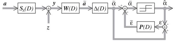
Fig. 10. Equivalent discrete-time system model of the MNP-DDFE.
