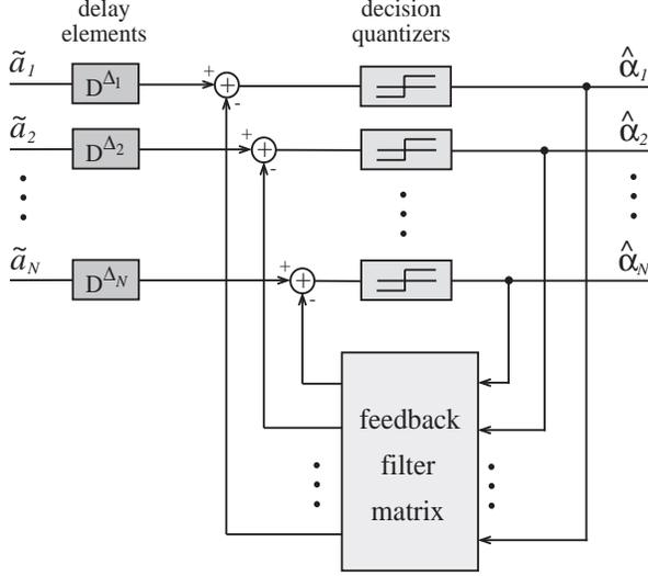
Fig. 8. Nonlinear decision device (NDD) of the M-DDFE.
