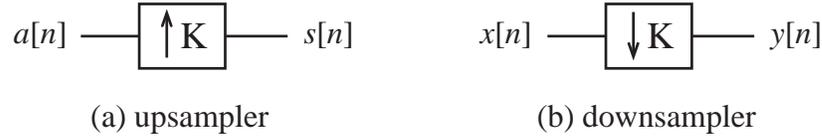
**Figure B.1:** Upsampler and downsampler symbol blocks.
