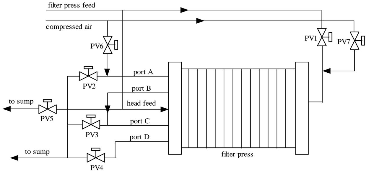
Figure 2.4.3 Filter Press System
