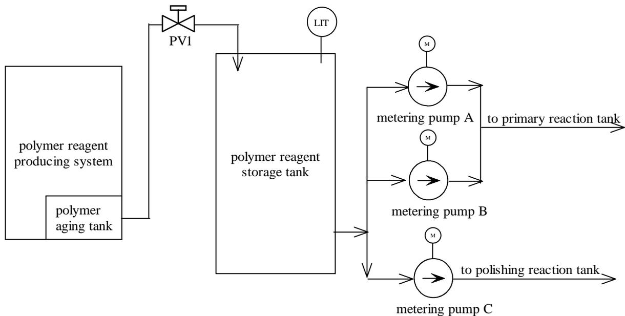
Figure 2.9.1 Polymer Reagent Preparation System
