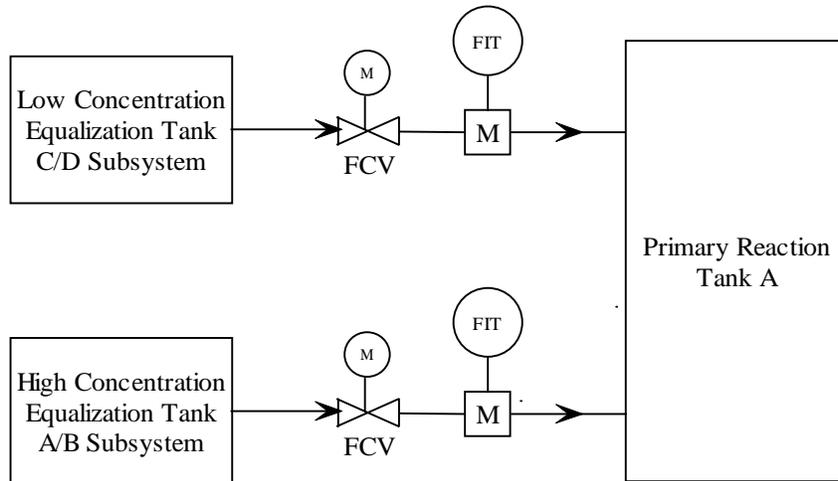
Figure 2.1.6 Equalization Tank to Primary Reaction Tank Feed Flow Rate Control
