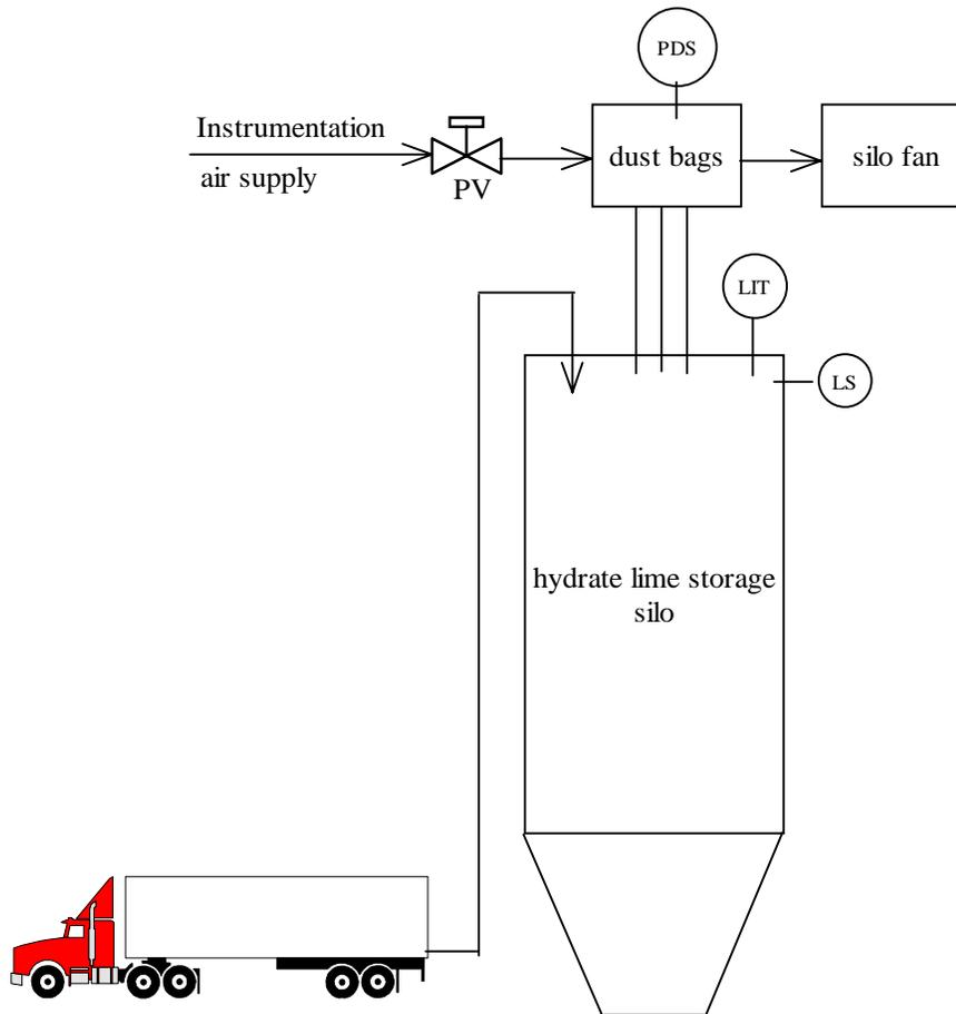
Figure 2.10.1 Lime Storage Silo System
