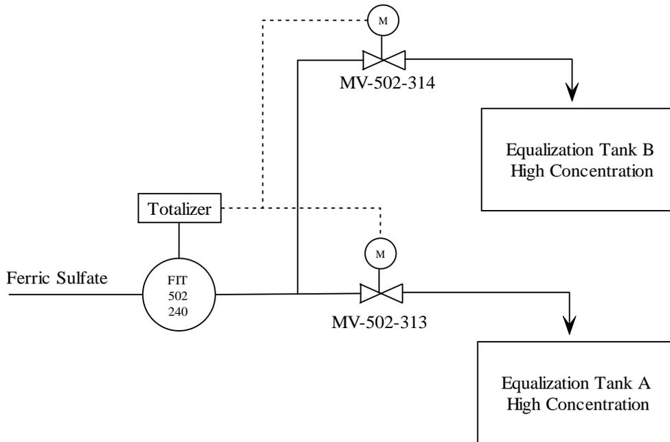
Figure 2.1.2 Equalization Tank Ferric Sulfate Addition
