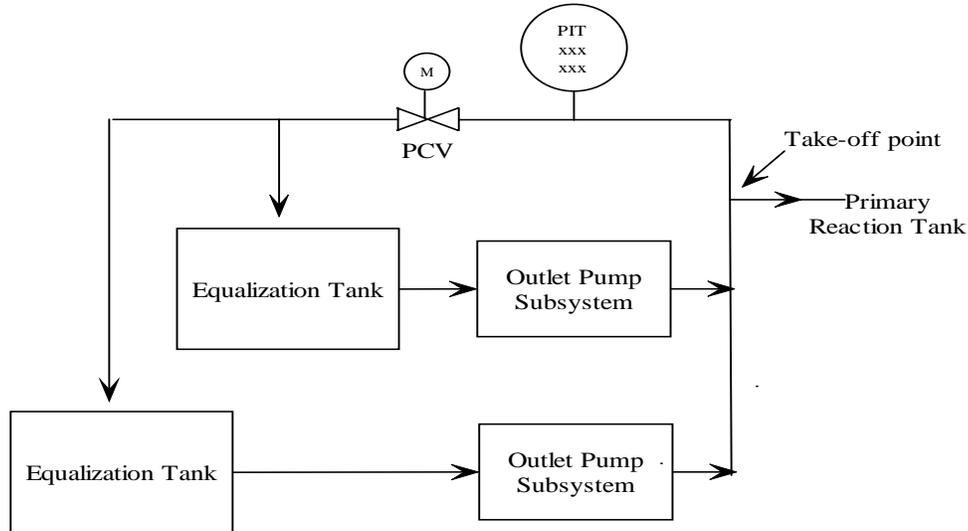
Figure 2.1.5 Equalization Tank Recycle Line Back Pressure Control
