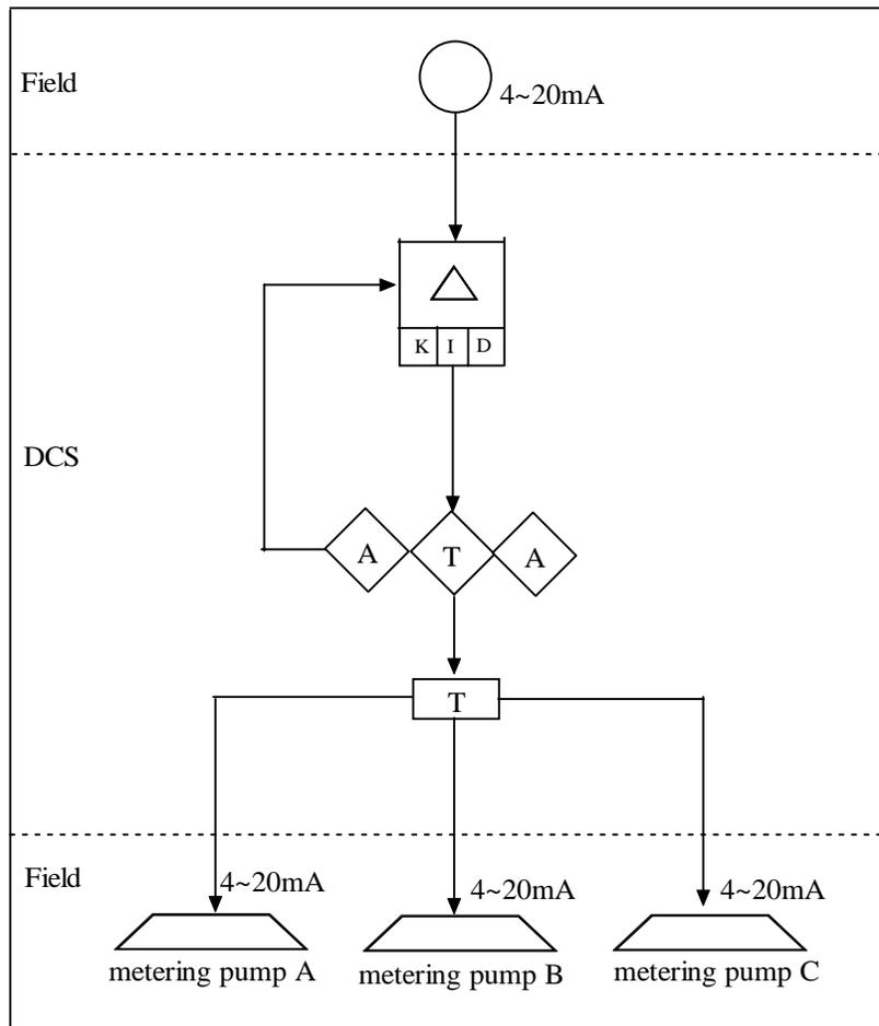
Figure 4.3.1 Polishing Reaction Tank Level Control
