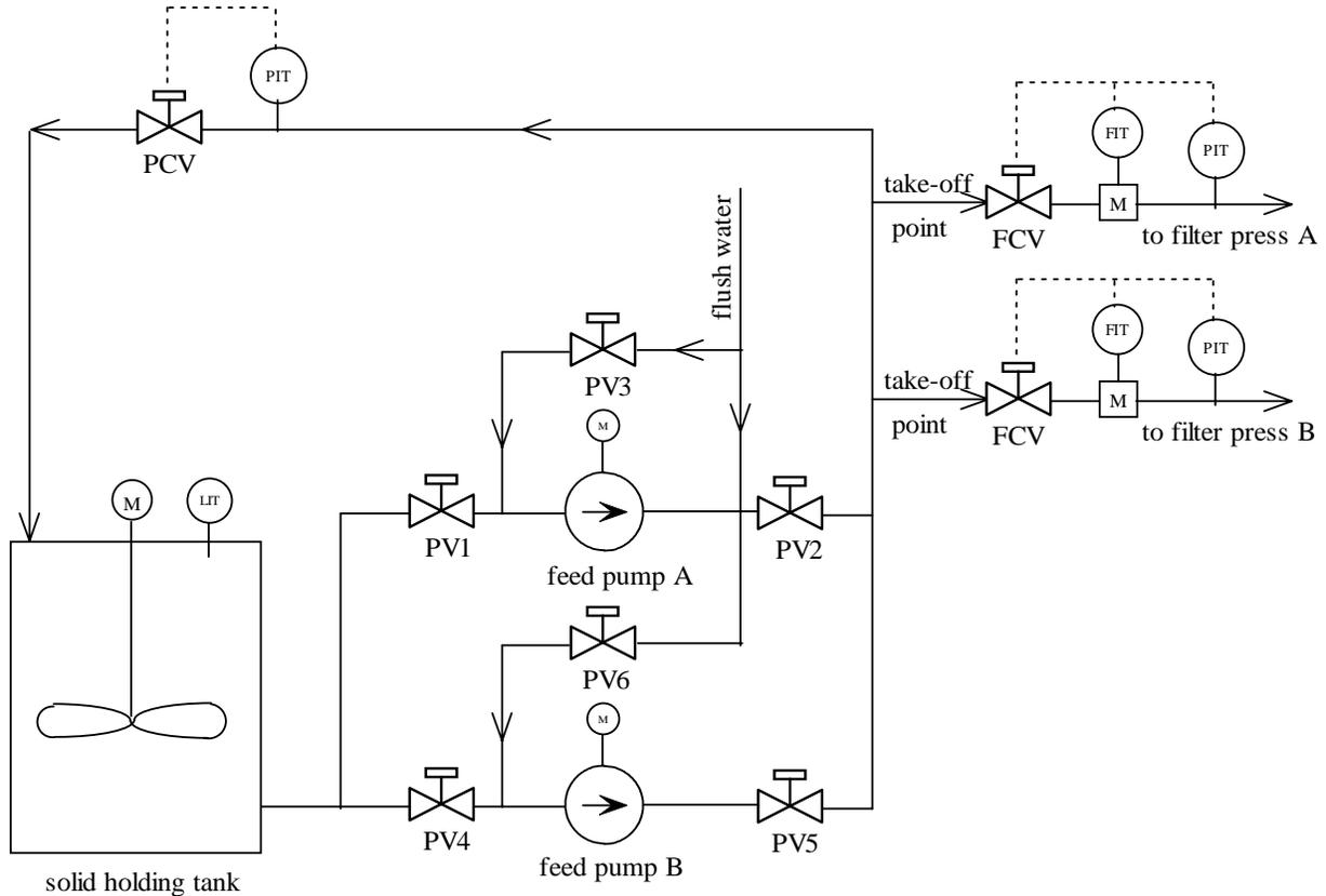
Figure 2.4.1 Filter Press Feed System
