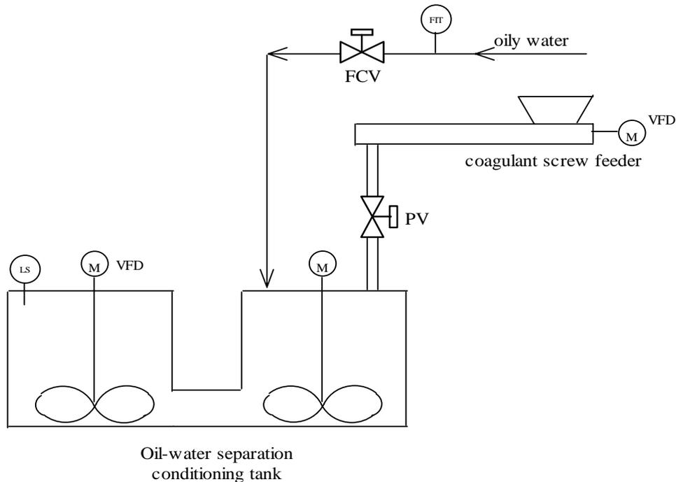
Figure 2.11.3 Coagulant Solution Preparation and Addition System
