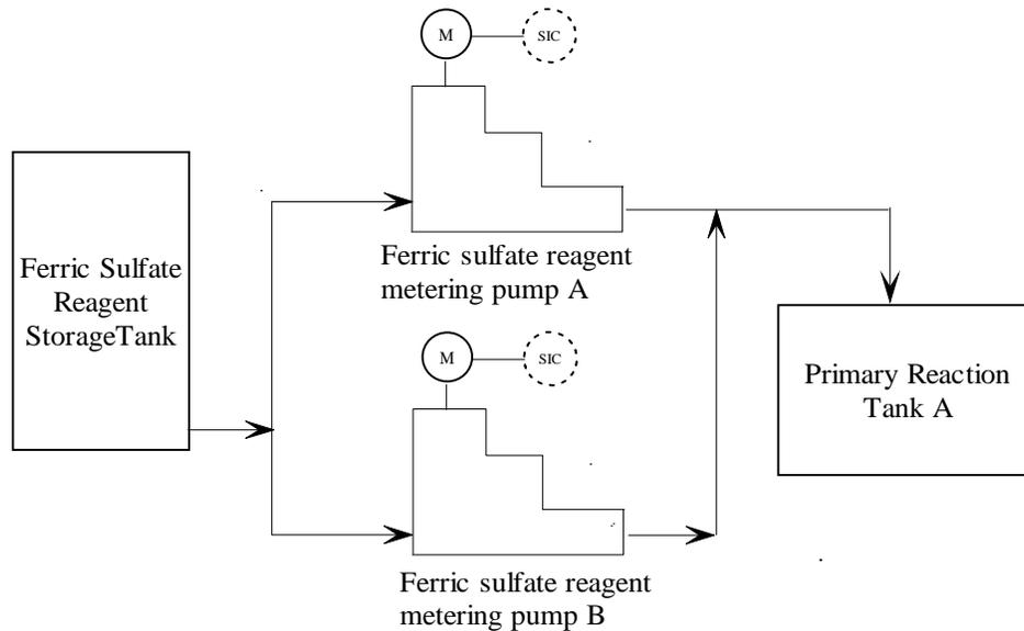
Figure 2.2.3 Primary Reaction Tank A ferric sulfate solution addition
