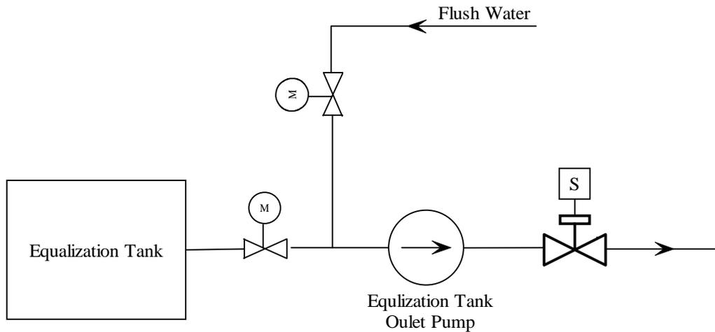
Figure 2.1.4 Equalization Tank Outlet Pump
