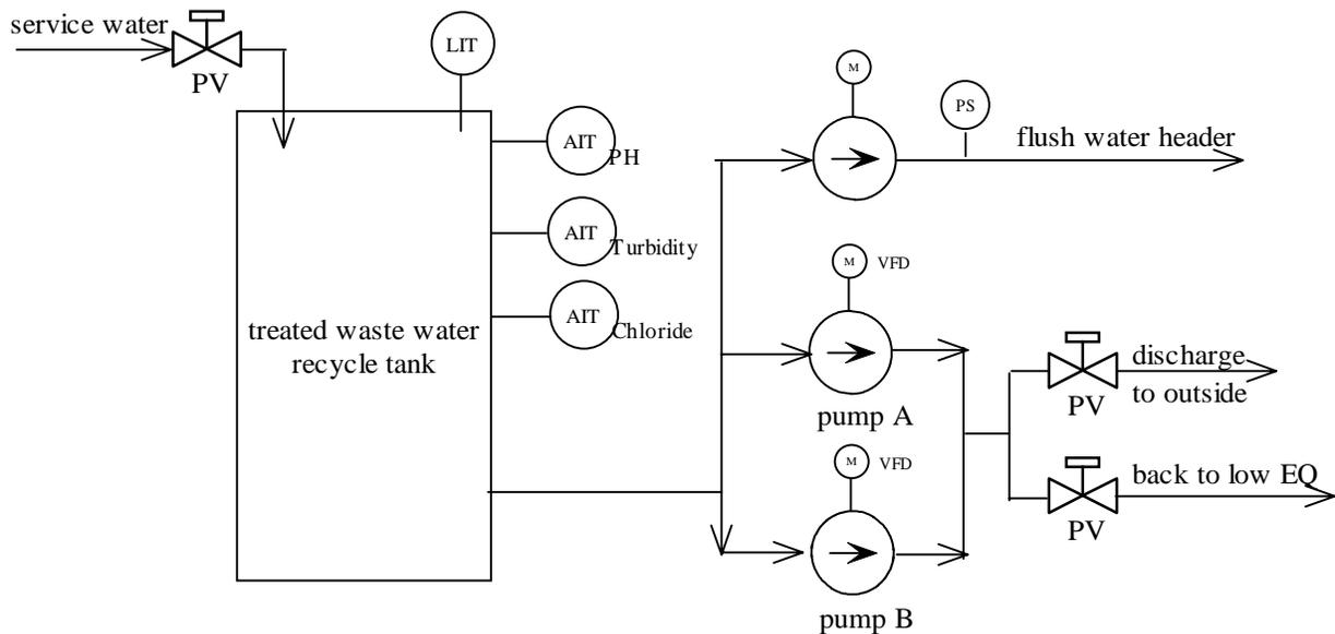
Figure 2.7.1 Treated Waste Water Recycle System
