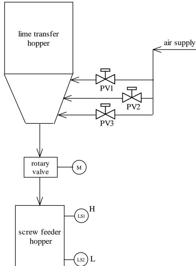
Figure 2.10.3 Lime Transfer from Transfer Hopper to Screw Feeder Hopper System
