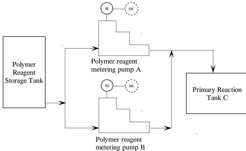
Figure 2.2.5 Polymer solution addition
