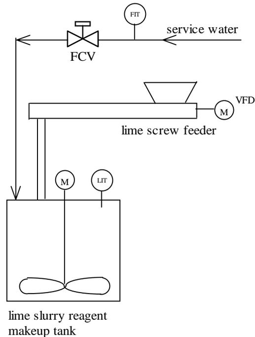
Figure 2.10.4 Lime Slurry Producing System
