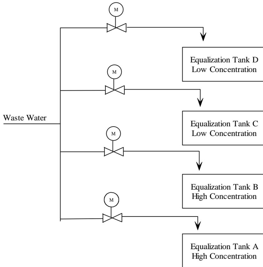
Figure 2.1.1 Equalization Tank incoming waste water
