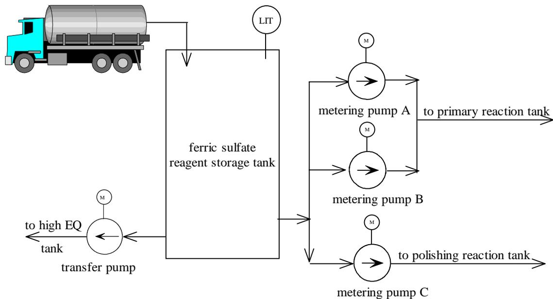
Figure 2.8.1 Ferric Sulfate Reagent Preparation System
