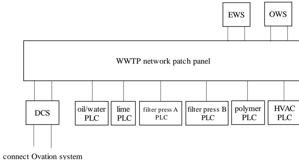
Figure 3.1.1 Control System Architecture
