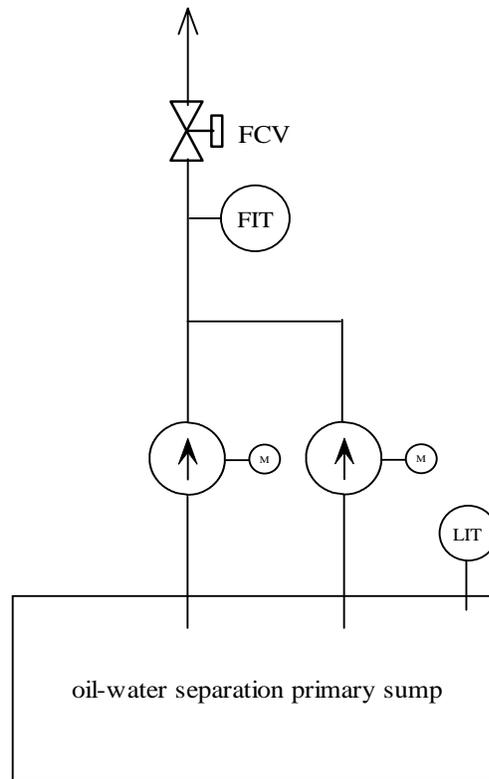
Figure 2.11.4 OWS Cartridge Filter Feed System
