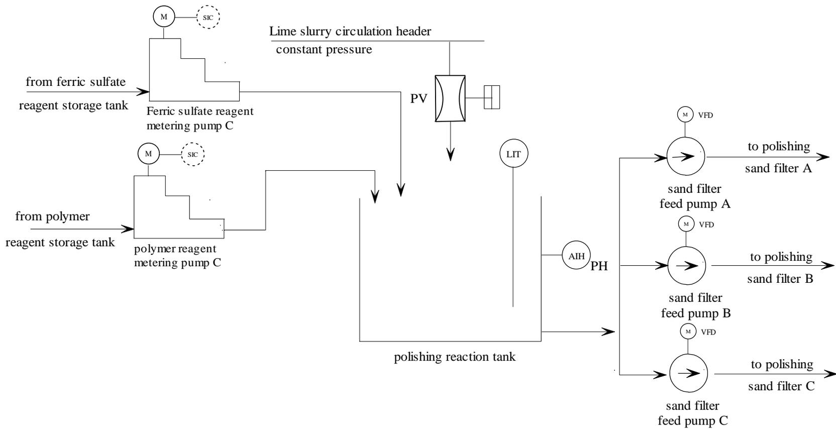
Figure 2.5.1 Polishing reaction system
