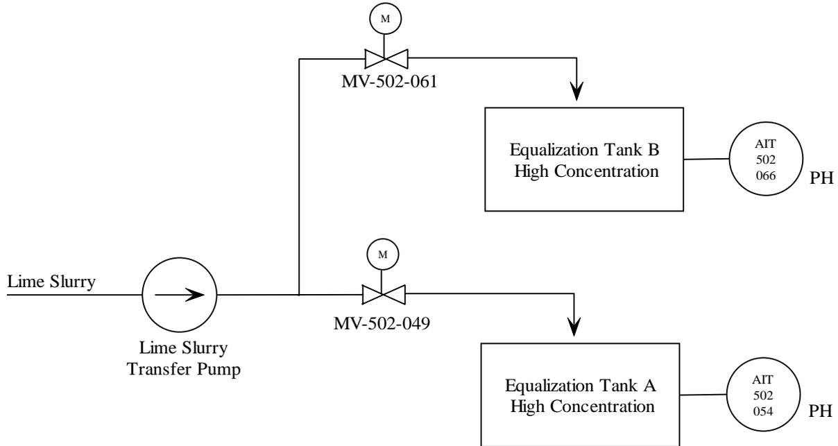
Figure 2.1.3 Equalization Tank Lime Slurry Addition
