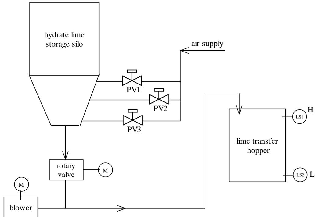
Figure 2.10.2 Lime Transfer from Silo to Hopper System
