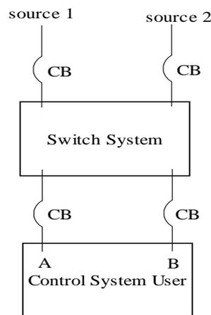
Figure 3.1.1 WWTP Power System for Control Use
