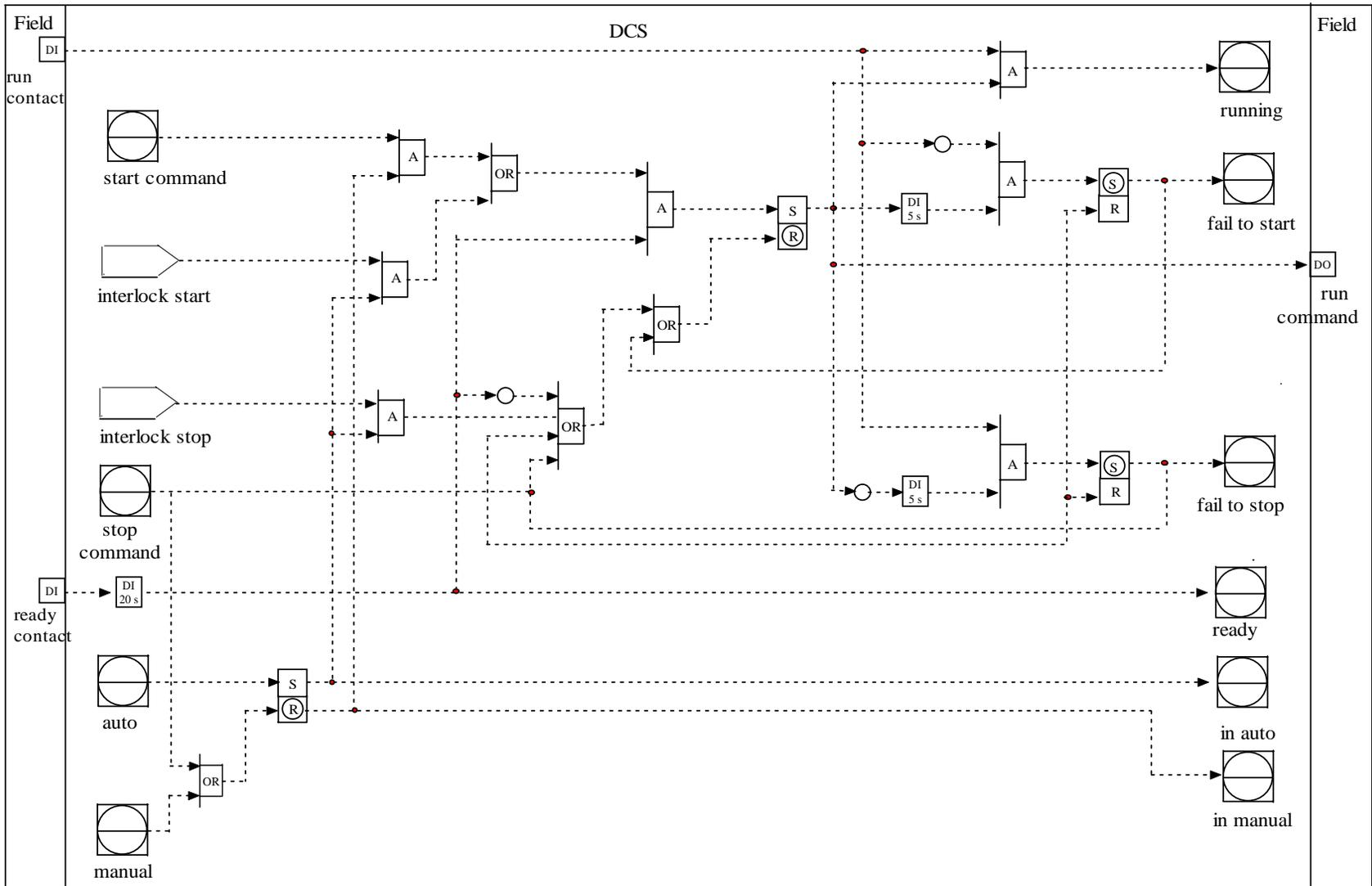
Figure 4.1.1 Agitator control logic
