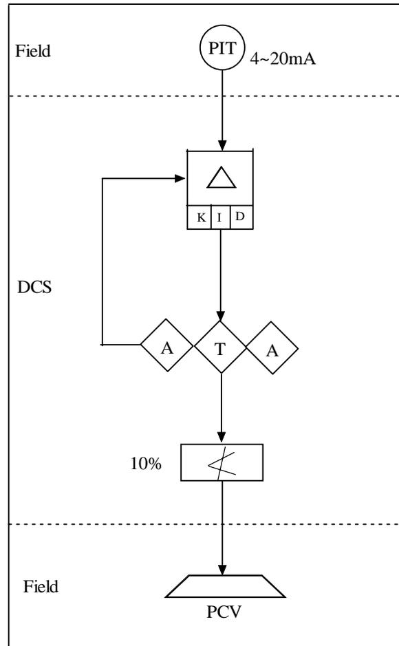
Figure 4.2.1 Back Pressure Loop Control
