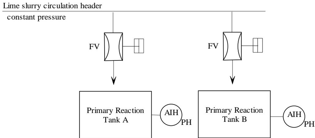
Figure 2.2.1 Primary Reaction Tank A and B lime solution addition
