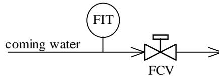
Figure 2.11.2 Incoming Water Flow Control System
