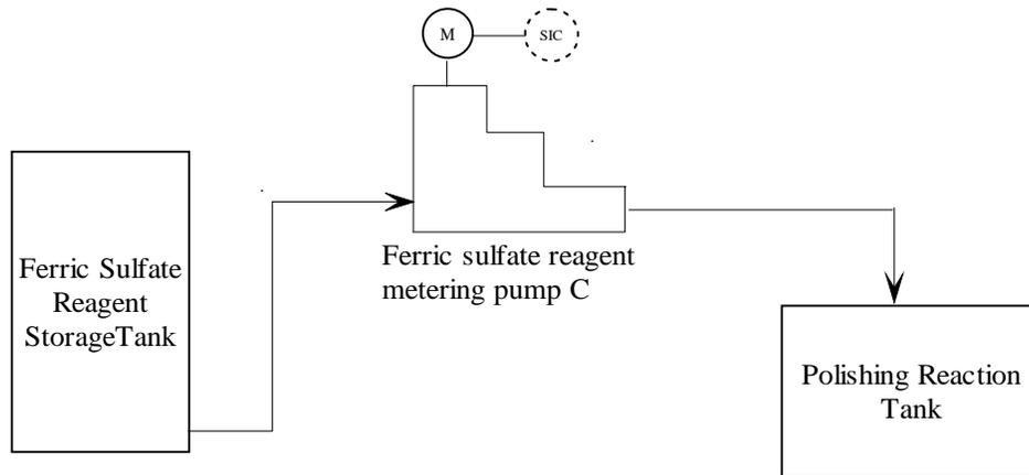
Figure 2.2.3 Polishing Reaction Tank ferric sulfate solution addition
