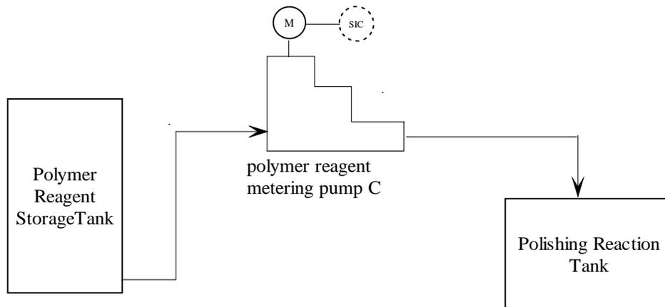
Figure 2.2.5 Polishing reaction tank polymer solution addition
