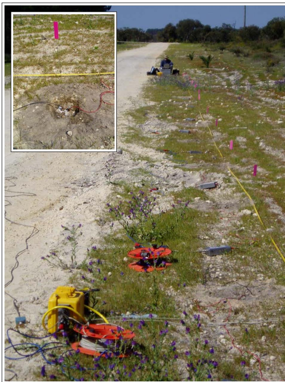
Figure A.2: Seismoelectric instrumentation consisting of preamplifiers (silver boxes), Geode seismograph (yellow box) and recording computer (in background) deployed along Cypress Rd. near borehole P-90 (Western Australia). The inset image shows a typical foil electrode used during that survey.
